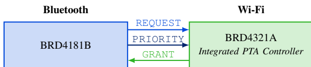
Fig. 8: PTA implementation by Silicon Labs .
