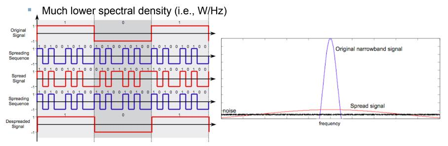
Benefits: anti-jamming, anti-interference, possible low probability of detection/intercept, uncoordinated frequency reuse (e.g. CDMA)
